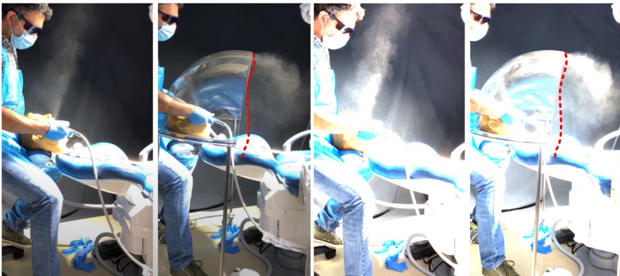
Figure 4: Dentist exposure to the aerosol cloud (with and without barrier)
